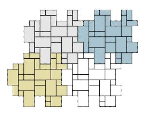
$\label{layer} \mbox{Pacific-Eco pallet layer for conventional install. Pattern uses one full layer.}$
